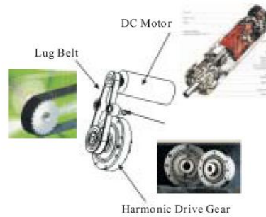
Figure 7: Drive system of WABIAN-2
